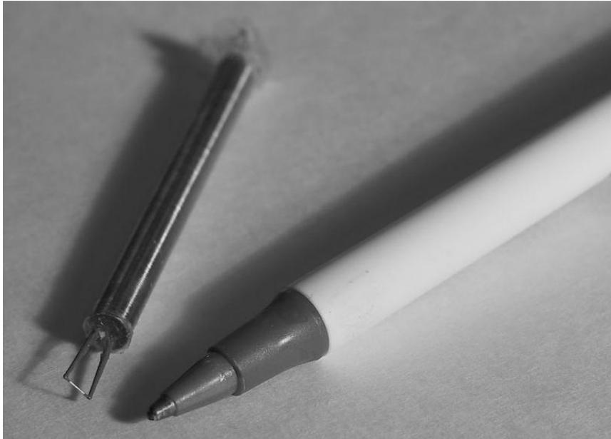
**Figure 3.8:** Photo of a hot-film probe. The sensing element is 3 mm long and  $25\ \mu\text{m}$  in thickness.
