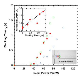
FIG. 2. (Color online) Dependence of the blocking time  $\tau_b$  on laser power and position (indicated in the picture) for  $Q_{\rm water} = 0.03~\mu \rm L/min$  and  $Q_{\rm oil} = 0.1~\mu \rm L/min$ ,  $\omega_0 = 2.6~\mu \rm m$ . Inset: Rescaled droplet length  $L/L_0$  vs the blocking time (laser position •), where  $L_0$  is the droplet length without the laser. The dashed line is a linear fit, ignoring the outlier at  $\tau_b = 0.75~\rm s$ .
