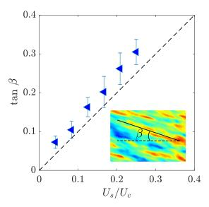
FIG. 6. Tilt angle  $\beta$  of the wrinkles in a transverse current at fixed Reynolds numbers Re<sub>\delta</sub> = 550 as a function of  $U_s/U_c$ . Each point is obtained by fitting straight lines through the surface deformation patterns and averaging over a large number of realizations. The dashed line is the geometric prediction  $\tan \beta = U_s/U_c$ , with  $U_c \simeq 12u^*$  the convection velocity of the pressure fluctuations.
