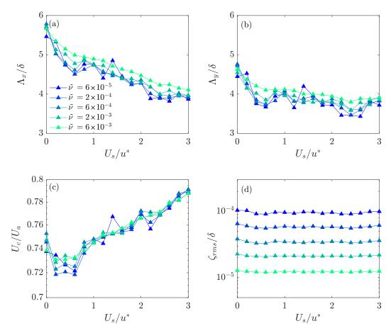
FIG. 9. Modification of the wrinkle properties for a longitudinal current as a function of  $U_s/u^*$ : Characteristic streamwise  $\Lambda_x/\delta$  (a) and spanwise  $\Lambda_y/\delta$  (b) lengths, convection velocity  $U_c/U_a$  (c), and wrinkle amplitude  $\zeta_{\rm rms}/\delta$  (d). Results are obtained for Re $_\delta=100$  in the large DNS box ( $60\pi$ ,  $6\pi$ ), with liquid viscosity varied in the range  $\tilde{v_\ell}=6\times 10^{-5}-6\times 10^{-3}$ .
