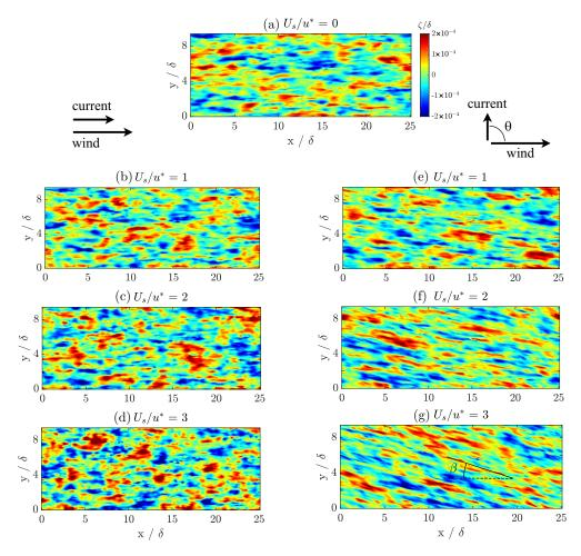
FIG. 5. Surface deformations without (a) and with (b–g) current. Snapshots are compared for increasing current  $U_s$  in the range  $(1-3)u^*$ , for a uniform current in the longitudinal (b–d) and transverse (e–g) directions ( $\theta = 0$  and  $\theta = \pi/2$ , respectively). Results are shown for Re<sub> $\delta$ </sub> = 350 and a liquid viscosity  $\tilde{v}_{\ell} = 6 \times 10^{-3}$ .
