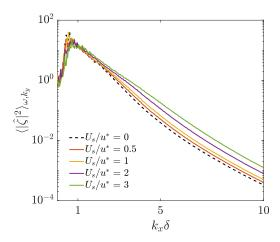
FIG. 8. One-dimensional energy spectrum  $|\hat{\zeta}|^2$  of the surface deformation averaged over  $\omega$  and  $k_y$  for increasing current  $U_s$  in the longitudinal direction. Results are obtained for  $\text{Re}_{\delta} = 100$  in the large DNS box  $(60\pi, 6\pi)$  with liquid viscosity  $\tilde{v}_{\ell} = 6 \times 10^{-3}$ .
