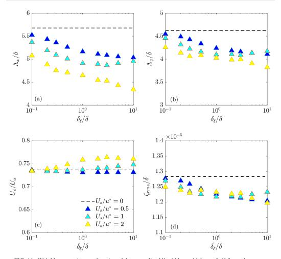
FIG. 11. Wrinkle properties as a function of the normalized liquid layer thickness  $\delta_{\ell}/\delta$  for various currents  $U_s/u^*=0.5, 1, 2$ . Reference values obtained without any current ( $U_s=0$ ) are represented by the dashed black lines. Results are obtained at  $\text{Re}_{\delta}=100$  for the large box  $(60\pi, 6\pi)\delta$ , with a liquid viscosity of  $\tilde{v}_{\ell}=6\times 10^{-3}$ .
