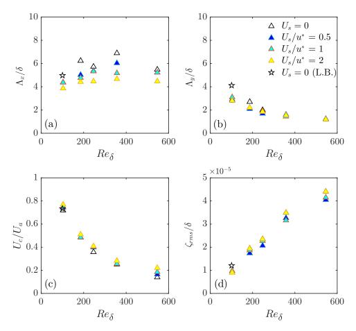
FIG. 10. Wrinkle properties as a function of the Reynolds number  $\text{Re}_{\delta}$  for three different currents  $U_s/u^*$  and a liquid viscosity  $\tilde{v}_{\ell} = 6 \times 10^{-3}$ . Results are obtained using the spectral interpolation method described in Sec. III.  $\Delta$ : small box, for various values of  $U_s/u^*$ ;  $\star$ : large box (L.B.), for  $U_s = 0$  only.
