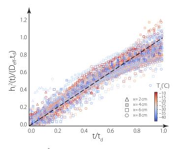
FIG. 3. Rescaled ice thickness  $h_i^2(t)/(D_{\text{eff}}t)$ ,  $t \in [0, t_d]$  as a function of the nondimensional time  $t/t_d$ .  $D_{\text{eff}}$  is computed from [17] and  $t_d$ , the time where the spatially homogeneous growth ends, is experimentally determined [see Fig. 2(a)].
