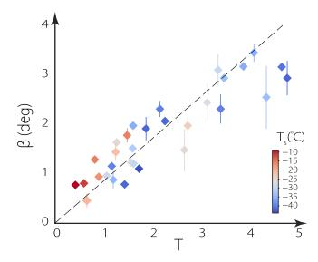
FIG. 4. Slope of the ice layer  $\beta$  as a function of the rescaled temperature  $\bar{T} = \frac{T_m - T_s}{T_{in} - T_m}$ . The dashed line is a linear fit of the data  $\beta = 0.77\bar{T}$ .
