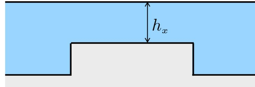
$$\nabla \cdot \left( \begin{pmatrix} h_x & 0 \\ 0 & h_y \end{pmatrix} \nabla \phi \right) - \frac{1}{g} \partial_{tt} \phi = 0 \quad h_x < \langle h^{-1} \rangle^{-1}, \quad h_y = \langle h \rangle$$
