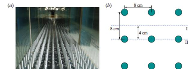
FIGURE 5. (Colour online) (a) Front view of the canopy. (b) Top view of the cylinder array. Station II marks the light sheet for photography.
