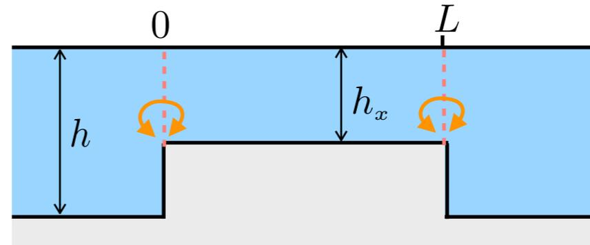
$$\nabla \cdot \left( \begin{pmatrix} h_x & 0 \\ 0 & h_y \end{pmatrix} \nabla \phi \right) - \frac{1}{g} \partial_{tt} \phi = 0 \quad h_x = \langle h^{-1} \rangle^{-1}, \quad h_y = \langle h \rangle$$
