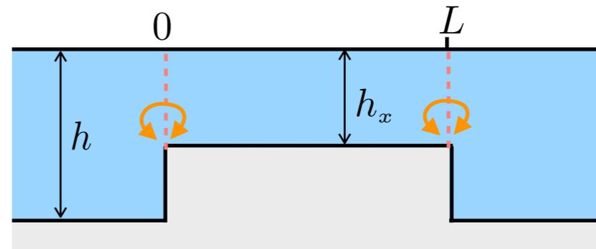
$$\nabla \cdot \left( \begin{pmatrix} h_x & 0 \\ 0 & h_y \end{pmatrix} \nabla \phi \right) - \frac{1}{g} \partial_{tt} \phi = 0 \quad \boxed{h_x = \langle h^{-1} \rangle^{-1}}, \quad h_y = \langle h \rangle$$
