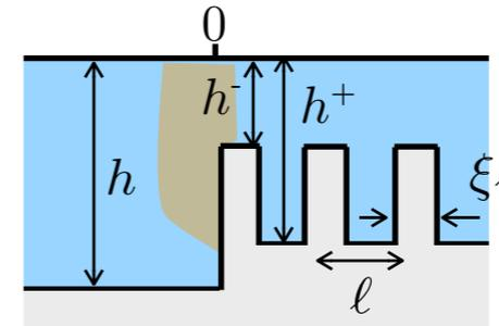
Main ingredients are: • rescaling :  $x \rightarrow x' = x/l$ ,  $y \rightarrow y$ ,  $z \rightarrow z' = z/h$ ,  $(x', z')$  micro scales
