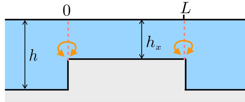
$$\nabla \cdot \left( \begin{pmatrix} h_x & 0 \\ 0 & h_y \end{pmatrix} \nabla \phi \right) - \frac{1}{g} \partial_{tt} \phi = 0 \quad \begin{matrix} h_x = \langle h^{-1} \rangle^{-1}, & h_y = \langle h \rangle \\ h_x < \langle h^{-1} \rangle^{-1}, \end{matrix}$$
