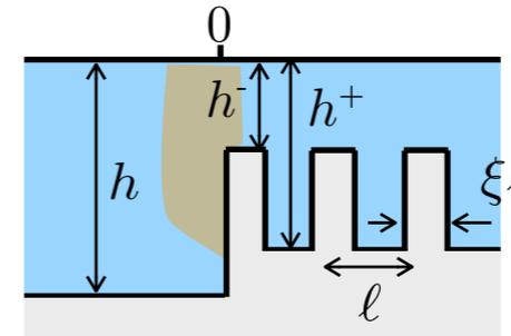
Main ingredients are: • rescaling :  $x \rightarrow x' = x/l$ ,  $y \rightarrow y$ ,  $z \rightarrow z' = z/h$ ,  $(x', z')$  micro scales
