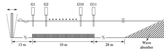
FIGURE 4. The set-up of the wave flume and canopy.
