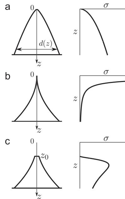
Fig. 7. The slender cone model: geometry and stress profile under uniform cross-flow. (a) cone with  $\beta < 1$  (here 0.75), showing a maximum of stress at the base; (b) cone with  $\beta > 1$  (here 2), showing a maximum at the top; (c) cone truncated arbitrarily at  $z_0=0.3$  showing a local maximum.
