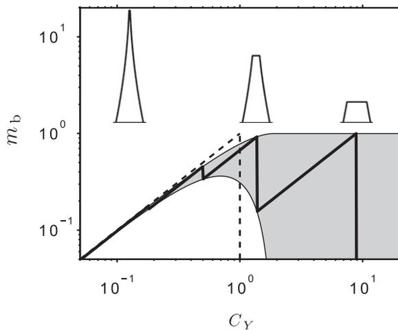
**Fig. 9.** Moment at the base of the cone as the fluid-loading is increased. (---) direct base breakage occurring when  $\beta < 1$ ; (—) progressive breaking for  $\beta > 1$  (here  $\beta = 2$ ). The shaded region shows all possible values depending on the initial truncation  $z_0$ . The cone state is shown for three values of  $C_Y$ .
