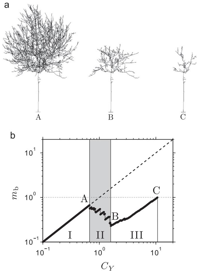
**Fig. 4.** Computed sequence of branch breakage in the walnut tree: (a) A: initial tree for  $C_Y \leq 0.67$ ; B: after breakage in large branches,  $C_Y = 1.7$ ; C: just before trunk breakage,  $C_Y = 10.7$ . (b) Corresponding evolution of the bending moment at the base of the tree  $m_b$ , in three distinct ranges. The dashed line shows the moment that would exist without breakage. The dotted line shows the critical value  $m_b$  that causes trunk breakage.
