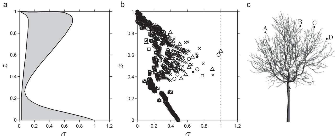
**Fig. 3.** Non-dimensional stress profile  $\sigma$  in a tree under cross-flow. (a) Schematic view of the stress profiles given by Niklas and Spatz (2000) for cherry trees, showing a local maximum near the top. (b) Computed stress profiles along four branching paths, A (x), B (□), C (△) and D (○) in the digitized tree geometry shown in (c).
