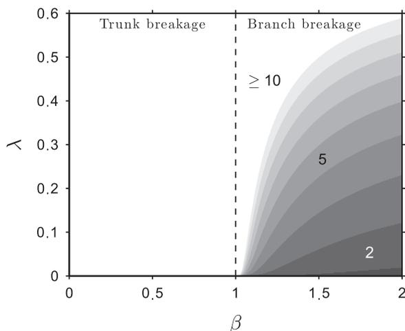
Fig. 6. Location of the maximum of stress under cross-flow in an idealized tree model, as a function of the slenderness exponent  $\beta$  and the branching parameter  $\lambda$ . The location is given in the form of the number of branching levels counted from the top of the tree, Fig. 5b. For  $\beta \leq 1$ , the breakage is directly at the base of trunk.
