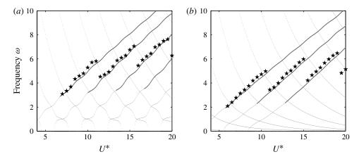
FIGURE 7. Evolution with  $U^*$  of the limit-cycle dominant frequency  $\omega$  (black star) for  $M^* = 10$ ,  $\alpha = 0.5$ , and (a)  $\beta = 0.03$ , (b)  $\beta = 0.31$ . In each case, the frequencies of the different linear modes are shown: light dotted lines correspond to stable modes and thick grey lines correspond to unstable modes. In each figure, from left to right, unstable frequencies correspond to flapping modes of increasing order and decreasing characteristic wavelength.
