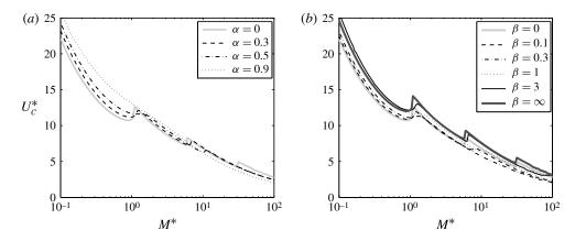
FIGURE 3. (a) Critical velocity threshold  $U_c^*$  as a function of the mass ratio  $M^*$  for  $\beta=1$  and varying  $\alpha$ . (b) Critical velocity threshold  $U_c^*$  as a function of the mass ratio  $M^*$  for  $\alpha=0.5$  and varying  $\beta$ .
