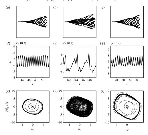
FIGURE 4. Limit-cycle oscillations: (a-c) flapping mode shape, (d-f) time-series of the non-dimensional harvested power  $\mathcal{P}(t)$  and (g-i) phase space trajectory for the trailing edge orientation  $\theta_e(t)$  for  $M^* = 10$ ,  $\alpha = 0.5$ ,  $\beta = 0.158$ , and (a,d,g)  $U^* = 10.5$ ,  $\eta = 3.8\%$ , (b,e,h)  $U^* = 11$ ,  $\eta = 1.7\%$  and (c,fi)  $U^* = 14.5$ ,  $\eta = 3.3\%$ .
