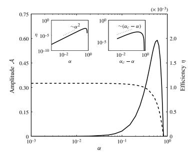
FIGURE 10. Evolution of the flapping amplitude  $\mathcal{A}$  (dashed) and harvesting efficiency  $\eta$  (solid) with the coupling coefficient  $\alpha$  for  $\beta=1$ ,  $M^*=0.5$  and  $U^*=15$ . The inset show the efficiency's scaling with  $\alpha$  in the limit of  $\alpha\ll 1$  and  $\alpha_c-\alpha\ll 1$  with  $\alpha_c\approx 0.82$  the critical value of  $\alpha$  leading to restabilization of the piezoelectric flag for those parameter values.
