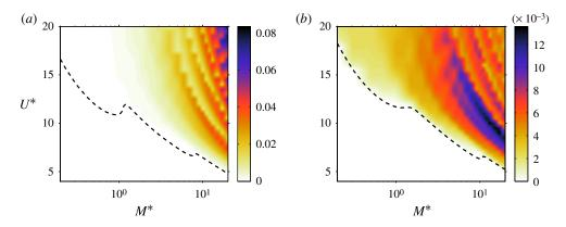
FIGURE 8. (Colour online) Harvesting efficiency  $\eta$  as a function of the mass ratio  $M^*$  and normalized velocity  $U^*$  for (a)  $\beta=0.1$  and (b)  $\beta=1$ . In both cases,  $\alpha=0.5$ . The black dashed line corresponds to the instability threshold  $U_c^*$ , below which  $\eta=0$ .
