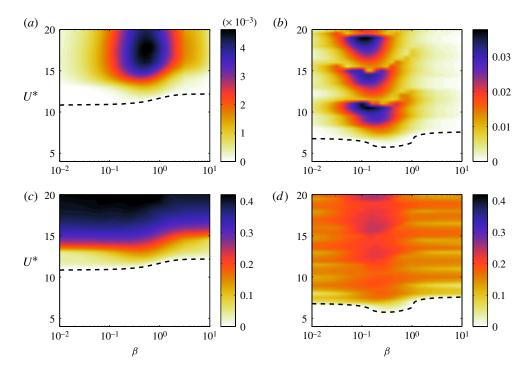
FIGURE 6. (Colour online) (a,b) Harvesting efficiency  $\eta$  and (c,d) flapping amplitude  $\mathcal{A}$  as a function of the tuning ratio  $\beta$  and the non-dimensional flow velocity  $U^*$  for (a,c)  $M^*=1$  and (b,d)  $M^*=10$ . For both cases,  $\alpha=0.5$ . The black dashed line corresponds to the instability threshold  $U_c^*$ , below which  $\eta=\mathcal{A}=0$ .
