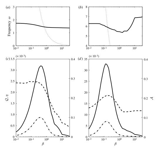
FIGURE 5. Evolution with the tuning ratio  $\beta$  of (a,b) the non-dimensional flapping frequency  $\omega$  and (c,d) the non-dimensional flapping amplitude  $\mathcal{A}$  (dashed), harvested energy  $\mathcal{Q}$  (dashedted) and harvesting efficiency  $\eta$  (solid) for  $\alpha=0.5$ ,  $U^*=14.5$ , and (a,c)  $M^*=1$ , (b,d)  $M^*=10$ . The dotted lines in (a,b) correspond to the variations of  $1/\beta$ .
