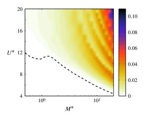
FIGURE 9. (Colour online) Harvesting efficiency obtained for the optimal tuning  $\beta$  as a function of the mass ratio  $M^*$  and non-dimensional velocity  $U^*$  for  $\alpha = 0.5$ . For each value of  $M^*$  and  $U^*$ ,  $\beta$  is chosen so as to maximize the harvesting efficiency. The black dashed line shows the minimum of the instability threshold over all possible values of  $\beta$ , below which  $\eta = 0$  for all  $\beta$ .
