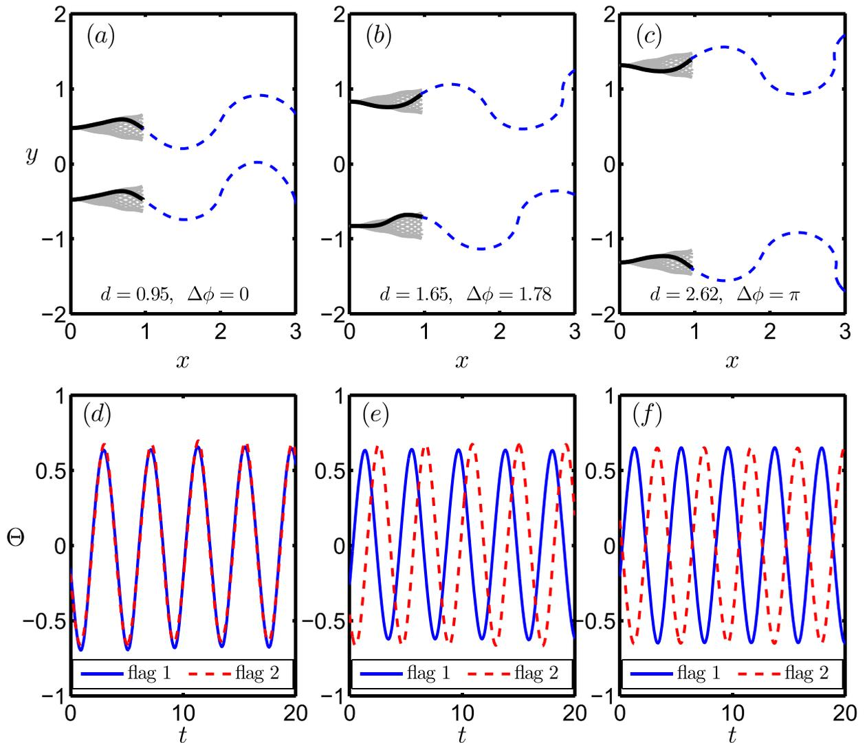
**Fig. 3.** (a,b,c) Flapping motion and instantaneous position of the flags and vortex sheets and (d,e,f) evolution of trailing edge deflection  $\theta_i$  in time for  $d=0.95$  (a,d),  $d=1.65$  (b,e) and  $d=2.62$  (c,f) for  $\alpha = 0$ ,  $M^* = 5$ ,  $U^* = 10$ .
