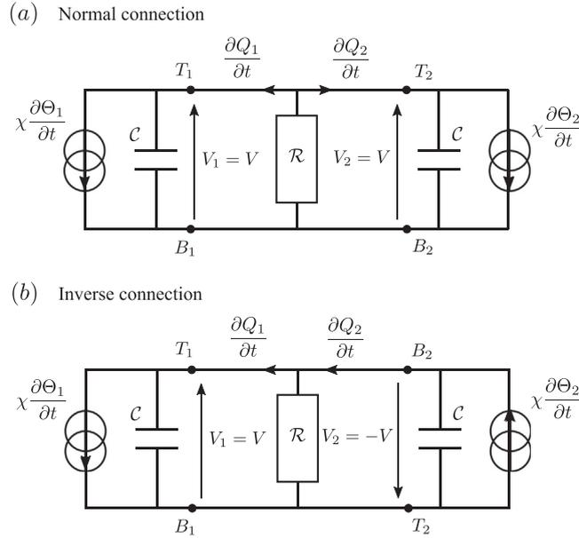
Fig. 2. Resistive circuit in (a) normal connection and (b) inverse connection.
