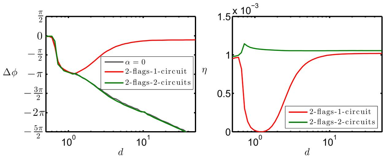
**Fig. 10.** (a) Phase shift  $\Delta\phi$  and (b) Harvesting efficiency  $\eta$  as function of  $d$  with two side-by-side flags and  $M^* = 3$ ,  $U^* = 13$  and  $\alpha = 0.3$ , connected in one circuit ( $\beta = 0.15$ ) and two isolated circuits ( $\beta = 0.31$ ). In (a), the phase shift obtained with  $\alpha = 0$  is also plotted for comparison.
