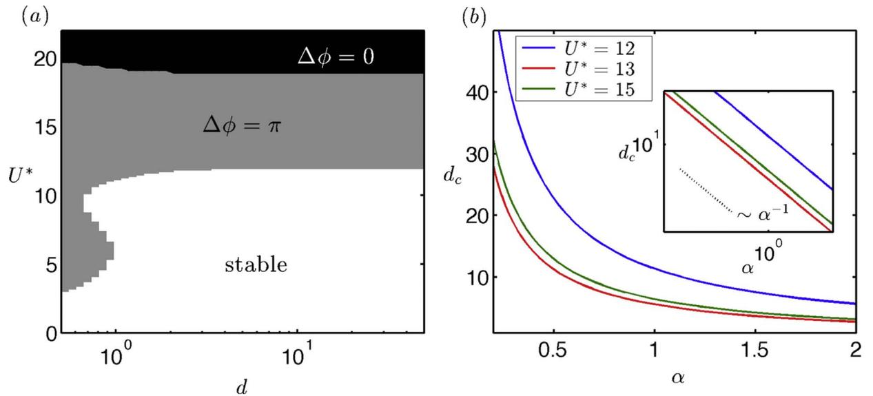
**Fig. 5.** (a) Relative phase of the two flags  $\Delta\phi$  in the most unstable mode as a function of  $d$  and  $U^*$ , for  $M^* = 3, \alpha = 0$  and  $\beta = 0.1$ . (b) Evolution with  $\alpha$  of the critical distance  $d_c$  at which the synchronization of the most unstable mode switches from out-of-phase to in-phase, for  $M^* = 3$  and varying  $U^*$ . The same data is plotted in logarithmic scale as an inset.
