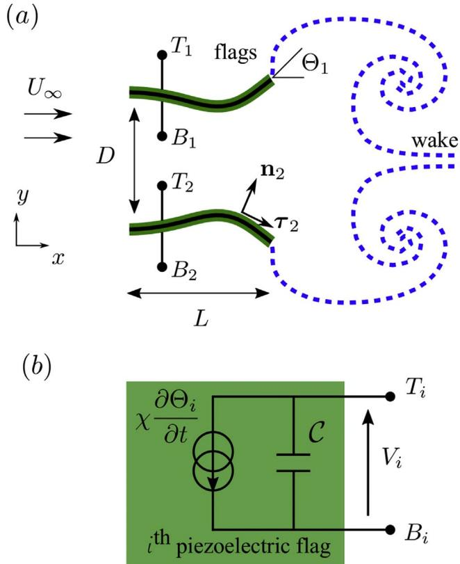
**Fig. 1.** (a) A schematic representation of two piezoelectric flags placed side-by-side in an axial flow, and (b) the electric equivalent of the *i*th piezoelectric flag with its two electrodes. The flags' electrodes are connected in a same circuit.
