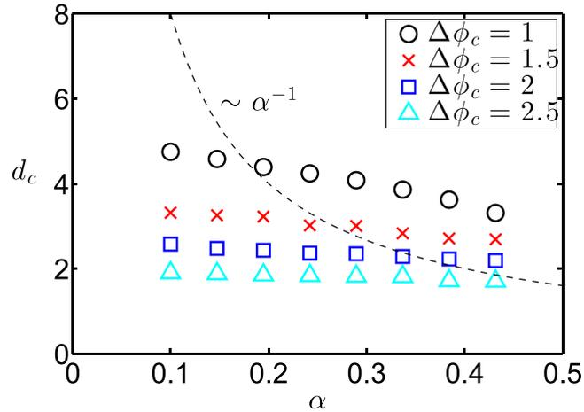
**Fig. 6.** Evolution with  $\alpha$  of the critical distance beyond which the phase difference between the flags is lower than  $\Delta\phi_c$ , for  $M^* = 3, U^* = 13$ . The linear result (Fig. 5) is also shown (dashed).
