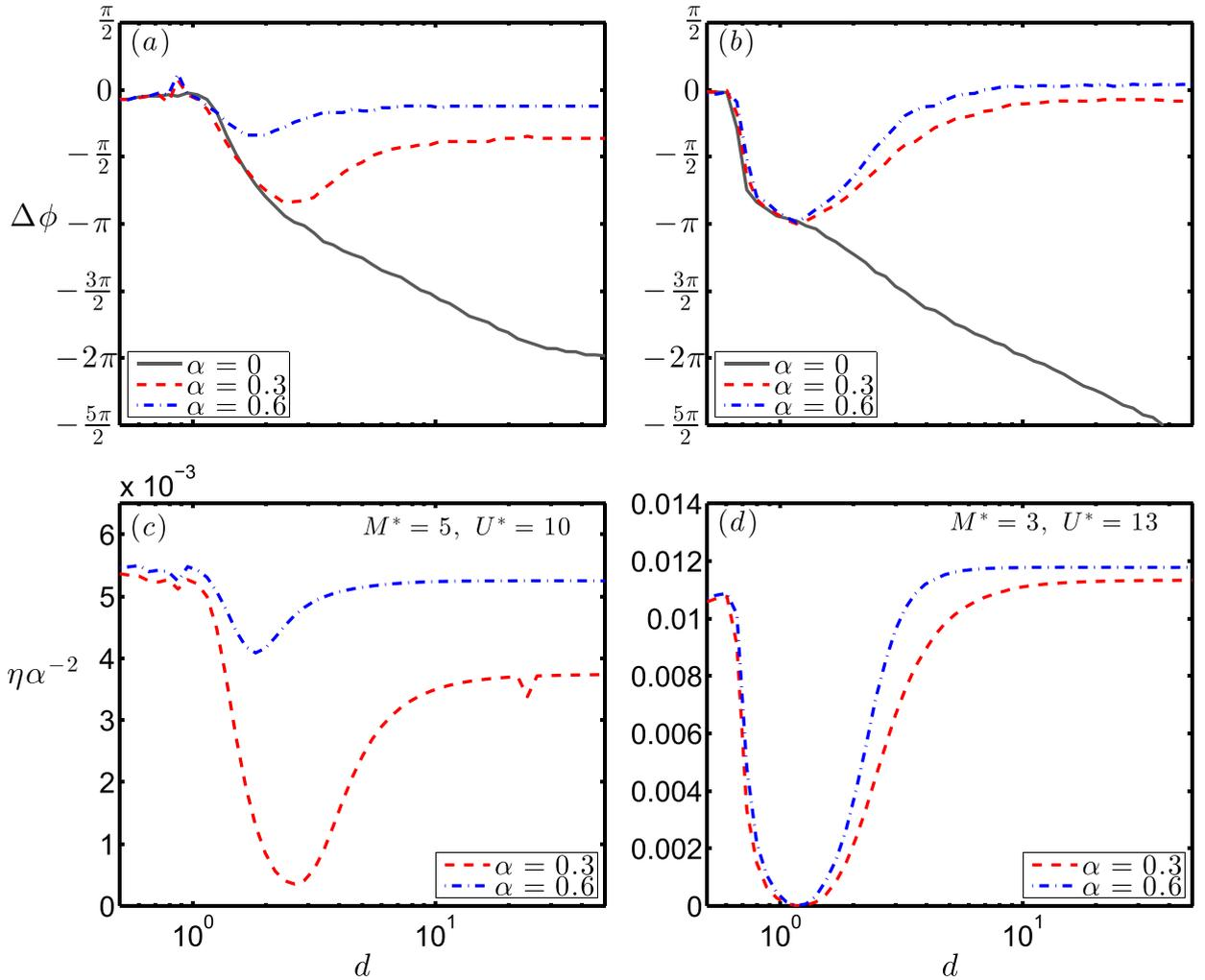
**Fig. 4.** Evolution with  $d$  of (a,b) the relative phase of the flags  $\Delta\phi$ , and (c,d) the rescaled harvesting efficiency  $\eta\alpha^{-2}$ , for  $M^* = 5, U^* = 10, \beta = 0.17$  (a,c) or  $M^* = 3, U^* = 13, \beta = 0.15$  (b,d).
