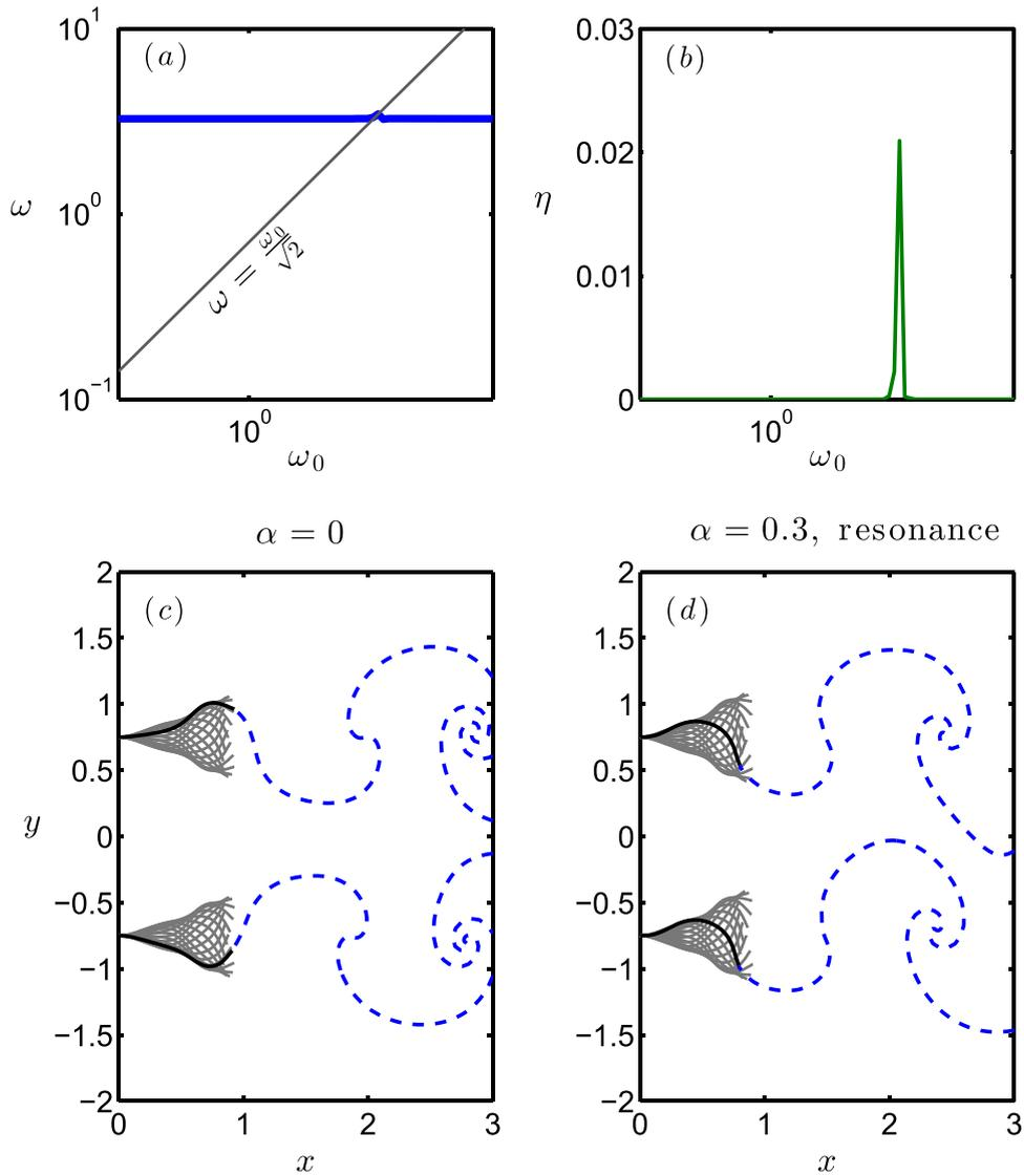
**Fig. 9.** (a) Flapping frequency  $\omega$  and (b) harvesting efficiency  $\eta$  with the normal connection,  $d=1.5$ ,  $\alpha = 0.3$ ,  $M^* = 3$ ,  $U^* = 13$ ,  $\beta = 10$ . Flapping motion of two flags with  $d=1.5$ ,  $M^* = 3$ ,  $U^* = 13$  and (c)  $\alpha = 0$ , (d)  $\alpha = 0.3$ ,  $\beta = 10$ ,  $\omega_0 = 4.88$ , normal connection at resonance.
