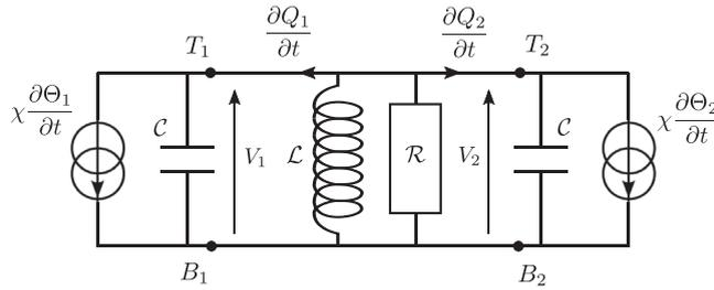
Fig. 8. Resistive-inductive circuit connected to two piezoelectric flags.
