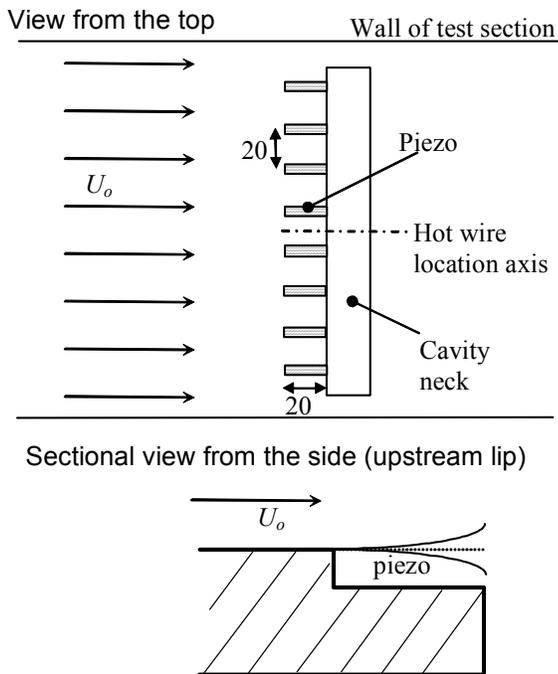
Figure 7. Sketch of the actuators mounting
