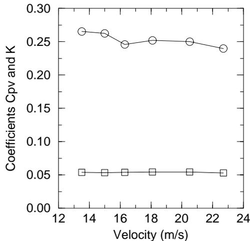
Figure 1. Mean pressure coefficients versus  $U_0$
