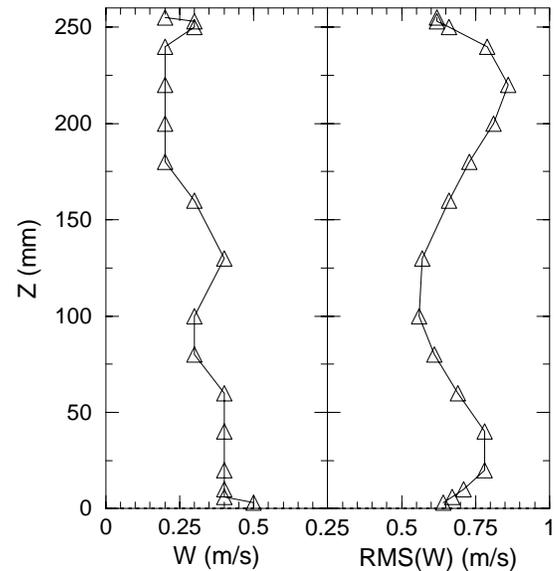
Figure 3. Profiles of vertical velocity  $W$  at  $X=-2L$  and  $U_0=15.7$  m/s
