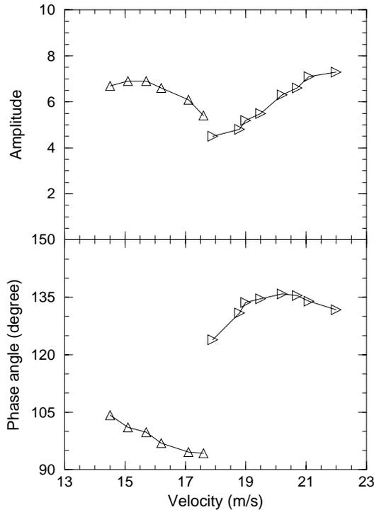
**Figure 6. Transfer function  $P_v/P_e$  versus  $U_o$  for the deep cavity**
