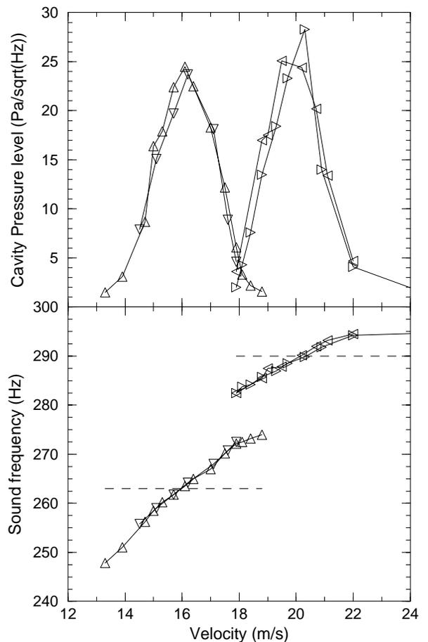
**Figure 4. Cavity pressure level and corresponding frequency versus  $U_o$  for the deep cavity**
