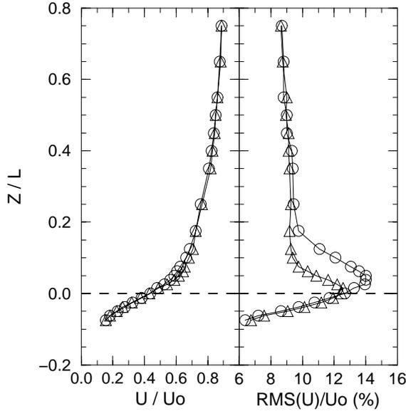
**Figure 9. Shear layer profile in the middle of the neck** ( $\Delta$ : without actuator,  $\circ$ : with all actuators at 310 Hz)
