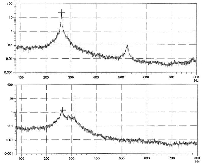
Figure 8. PSD of  $P_v$  for the first resonance. (upper: without actuator, lower: with all actuators at 310 Hz)
