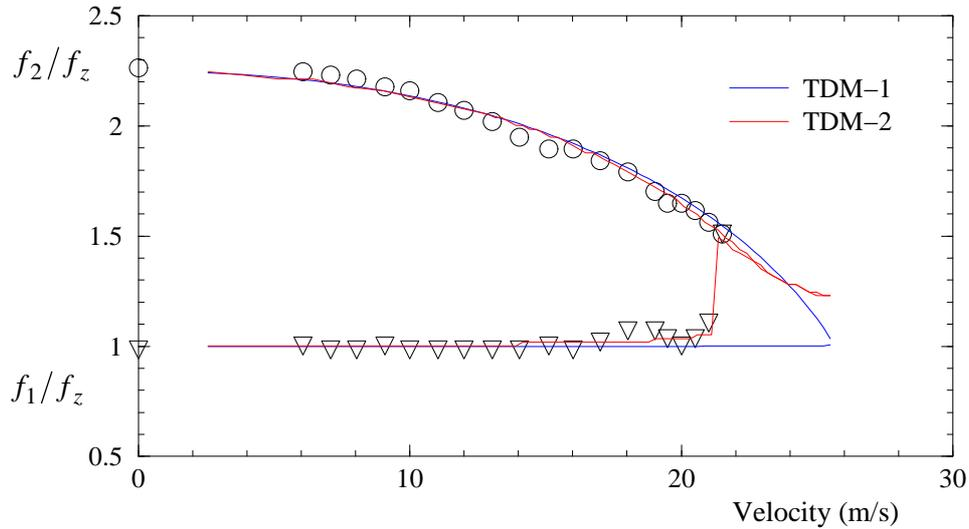
Figure 2: Evolution of frequencies versus wind velocity. Case B,  $U_c = 21.5$  m/s
