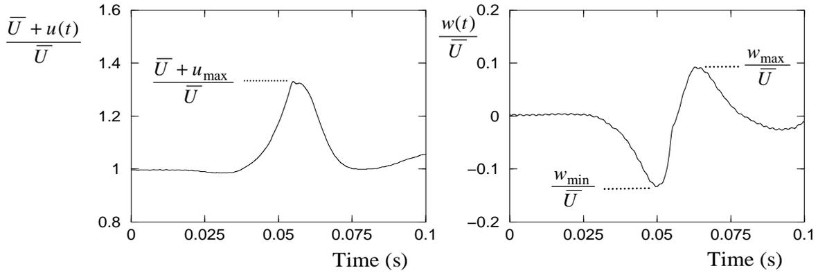
Figure 2: Sample of upstream velocity perturbation measured with a 2D hot wires probe.
