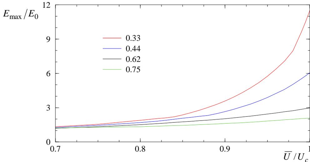
Figure 7: Effect of the frequency ratio on the maximum energy amplification versus velocity.
