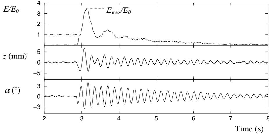
Figure 3: Typical transient response of the deck,  $\bar{U}/U_c = 0.91$ , Case A.
