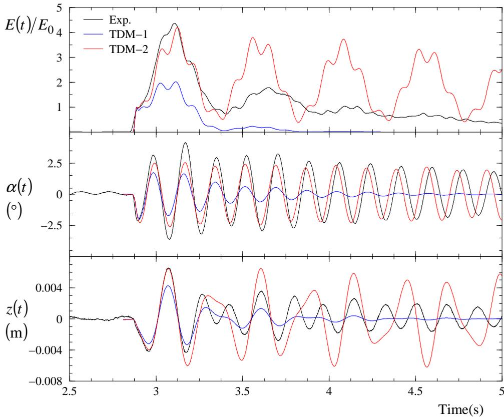
Figure 5: Time evolution of energy, angular displacement and vertical displacement.
