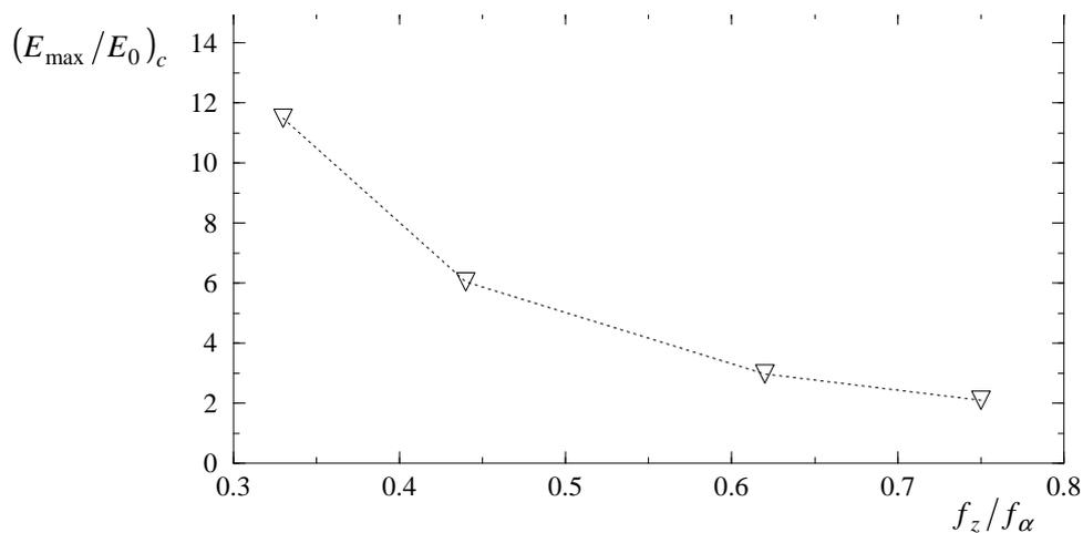
Figure 8: Influence of the frequency ratio on the maximum energy amplification at critical velocity.
