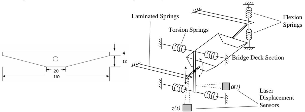
Figure 1: Bridge Deck Cross Section and Experimental Setup Schematics, dimensions in mm.
