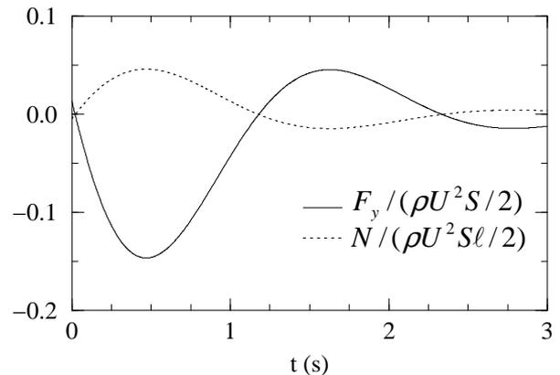
Figure 8. Transient evolution of the lateral force and yawing moment generated by an initial yawing rate,  $U=40$  m/s ( $U^*=0.89$ ), 3B vehicle.
