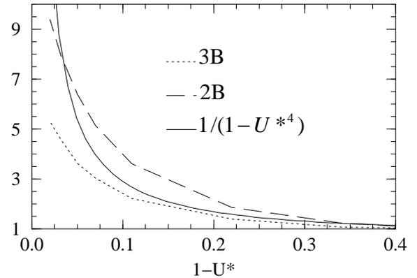
Figure 5. Maximum energy amplification versus velocity parameter for the two considered vehicles and comparison with the asymptotic law.
