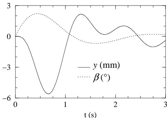
Figure 7. Transient evolution of the lateral displacement and yaw angle generated by an initial yawing rate,  $U=40$  m/s ( $U^*=0.89$ ), 3B vehicle.
