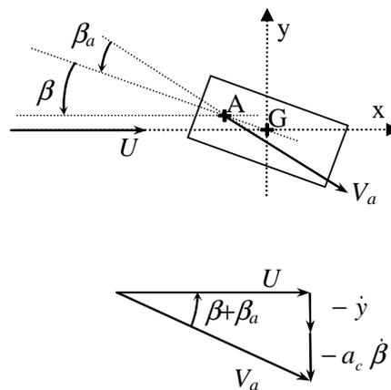
Figure 1. Definition of geometrical parameters and apparent velocity at point A
