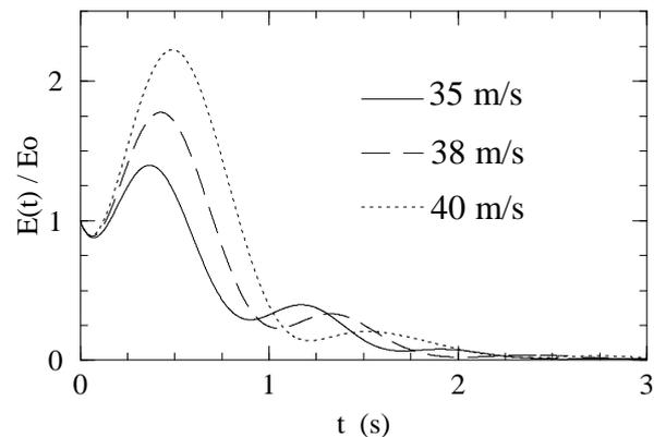
Figure 6. Influence of the free-stream velocity on the transient energy amplification with initial condition in yawing rate, 3B vehicle.
