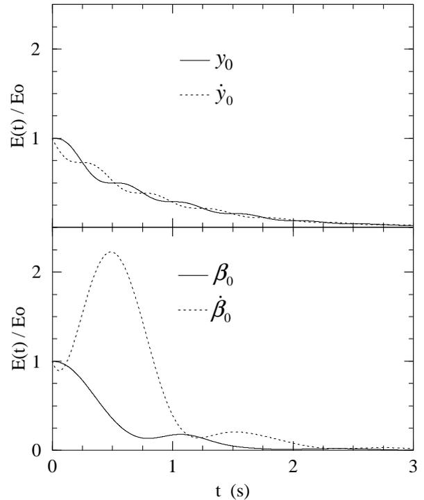
Figure 3. Transient energy amplification for various initial conditions,  $U=40$  m/s ( $U^*=0.89$ ), 3B vehicle.
