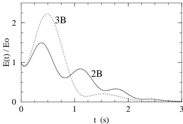
Figure 4. Comparison of the transient energy amplification between the two considered vehicles with initial condition in yawing rate,  $U=40$  m/s.
