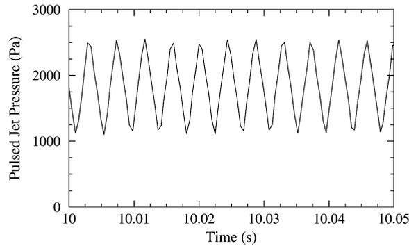
Fig. 3. Sample of time history of the pulsed jets pressure for a mean forcing pressure of 1 bar.
