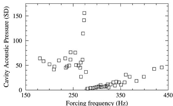
Fig. 8. Cavity pressure peak level versus forcing frequency at resonance ( $U_{ref} = 19.8$  m/s).
