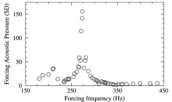
Fig. 10. Pressure peak level due to the actuators versus forcing frequency at resonant velocity ( $U_{ref} = 19.8$  m/s).
