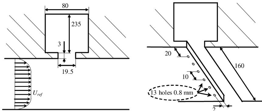
Fig. 1. Sketch of the cavity model showing the geometrical dimensions (mm).
