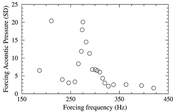
Fig. 11. Pressure peak level due to the actuators versus forcing frequency without wind ( $U_{\text{ref}} = 0$ ).
