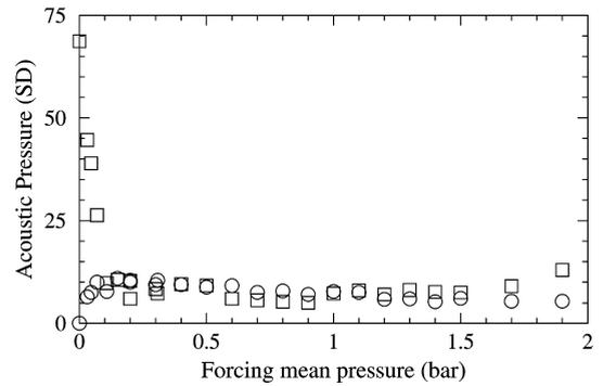
Fig. 12. Pressure peak level versus forcing pressure at resonant velocity ( $U_{\text{ref}} = 19.8$  m/s) and optimal forcing frequency ( $f_j = 316$  Hz).  $\square$ , cavity;  $\circ$ , actuators.
