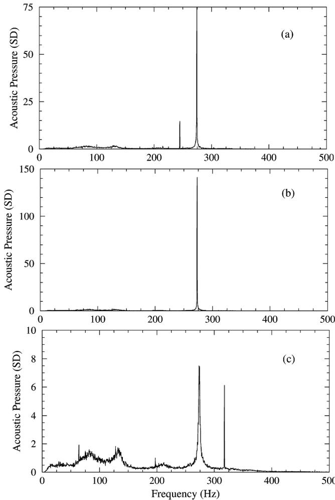
Fig. 9. Typical spectral densities of the acoustic pressure for three different forcing frequencies at resonance ( $U_{ref} = 19.8$  m/s). (a)  $f_j = 245$  Hz; (b)  $f_j = 272$  Hz; (c)  $f_j = 317.5$  Hz.
