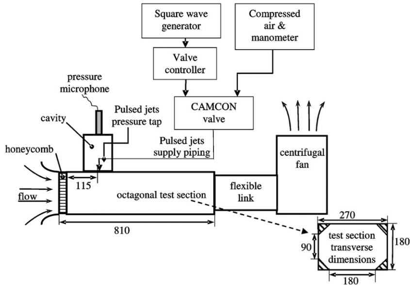
Fig. 2. Principle of the experimental setup.
