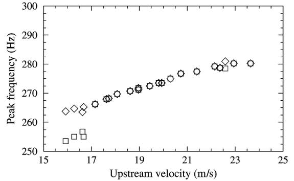
Fig. 5. Frequency of the pressure peak versus upstream reference velocity.
