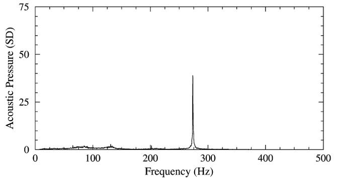
Fig. 7. Typical spectral density of the cavity acoustic pressure at resonance ( $U_{ref} = 19.8$  m/s).
