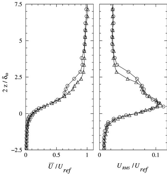
Fig. 4. Velocity profiles in the middle of the cavity neck at resonance ( $U_{ref} = 19.8$  m/s),  $\Delta$ : without forcing;  $\circ$ : with optimal forcing ( $f_j = 316$  Hz).
