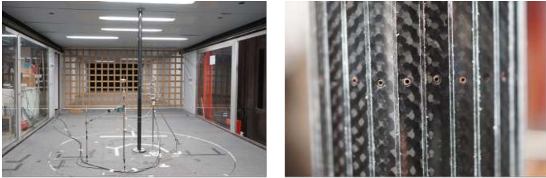
Figure 6: (a) Photo of the small scale cylinder in the test section and (b) detail of the measurement section equipped with pressure taps and ribs.
