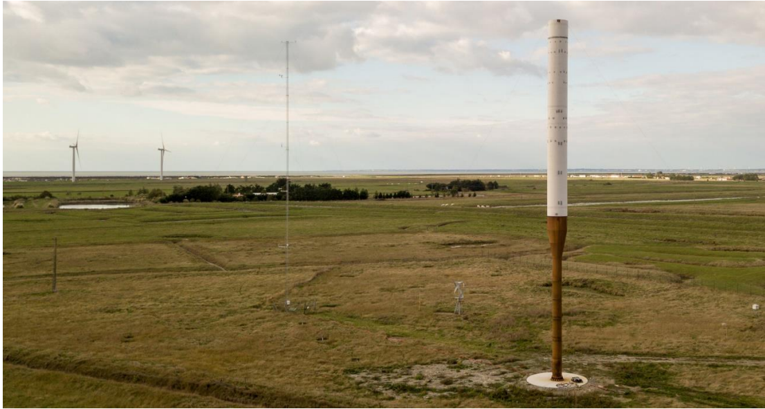
Figure 1 Experimental chimney in the monitored field (the mast with wind anemometers is slightly visible, see figure 2 for details).
