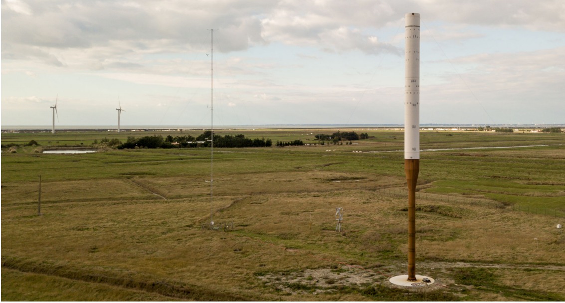
Figure 6.1: Experimental chimney in the monitored field with the wind anemometer mast slightly visible (see figure 2 for details). Photo by Lilian Vezin.
