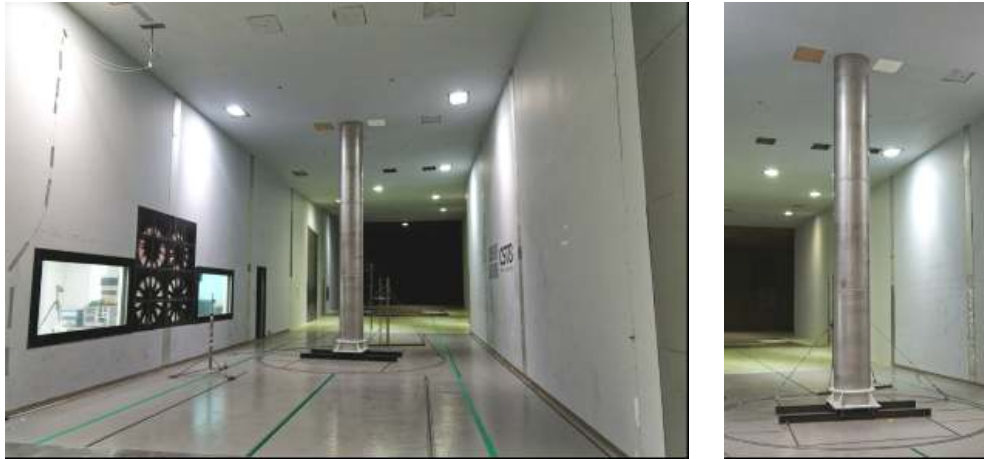
Figure 2: Views of the large 0.5 m diameter cylinder in the CSTB wind tunnel test section.
