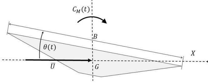
Figure 9: Studied configuration of bridge deck section
