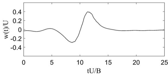
Figure 7: Gust velocity profile vs non-dimensional time
