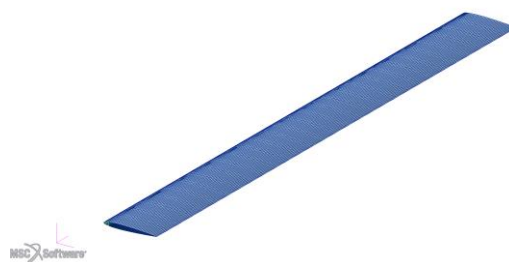
Figure 8: Finite element model of the wing for a flutter test.
