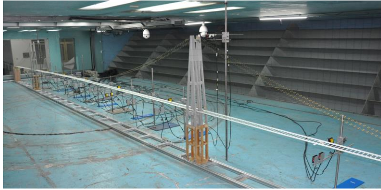
Figure 7: Full aeroelastic model of Taiwan Strait Bridge
