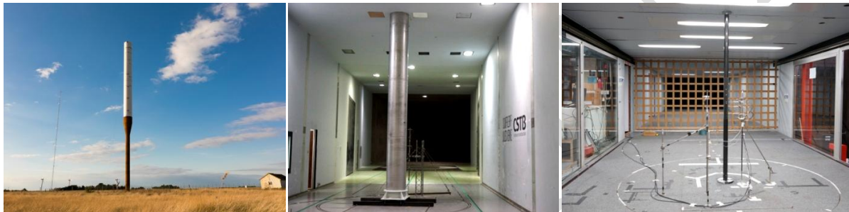
Figure 2. Views of the three experiments. From left to right: full scale chimney; large smooth cylinder in smooth flow; small rough cylinder in turbulent flow
