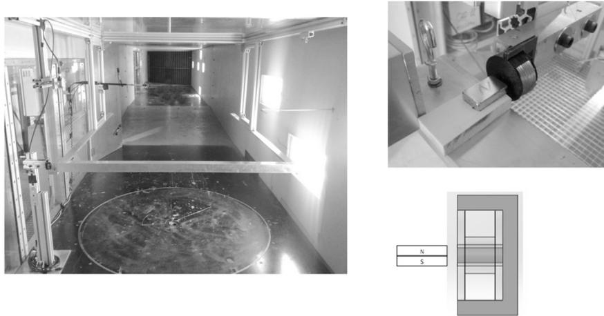
Fig. 2. Horizontal set-up installed in the test section (left) - Coil/magnet assembly (right).
