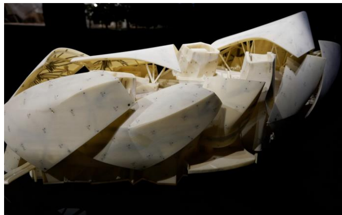
Fig. 3 The wind tunnel model of the Fondation Louis Vuitton, at scale 1/125
